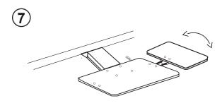
7. Press down to tilt the Mouse Pad and adjust its' angle. If the mouse pad is too loose, tighten the 2 screws on the mouse pad mounting bracket.
