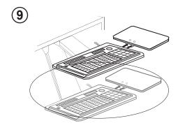
9. KTI is adjustable in height and angle. Release the lever (8A), adjust to your desired position, and lock the lever in place.
