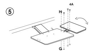
5. Connect the metal Mouse Pad Bracket to the keyboard tray using 2 H Screws & 2 G Nuts.
