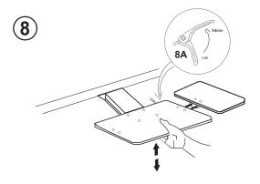
8. The Keyboard Tray slides in/out by pushing/pulling. 8A.To adjust the Keyboard Tray's angle, release the lever under the keyboard tray.
