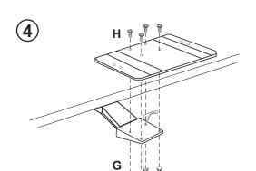
4. Attach the **Keyboard Panel (C)** to the mounting panel with 4 H Screws & 4 G nuts.
